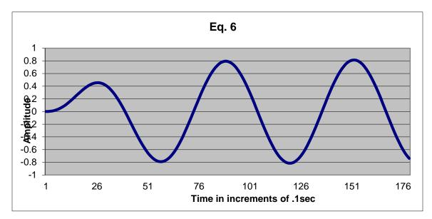
The graph of Eq. 6 illustrates the relationship between the impulse, or transient, response and the steady state response. It should be clear that while always a factor to be considered, the impulse response is short lived while the form of the steady state response mirrors the driver for this case. Filtering of non-sinus inputs will alter the form and amplitude of the output relative to the input, and we will cover some of those cases later in the series.
