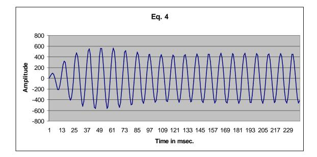
Bear in mind that  $v_L = L \frac{di}{dt} = i_L(j\omega L)$ , meaning that the magnitude of  $V_L$  is directly proportional to the magnitudes of both  $i_L \& \omega$ . The gross effect is that considerable voltage can be built across an inductor, which may present a hazard to the remaining circuitry. Of course there are techniques to control and/or limit the magnitudes, but that discussion is for a later time.
