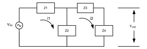
Writing the circuit equation for each loop; reveals that there are two equations in two unknowns ( $i_1 \& i_2$ ) that characterize the circuit.
