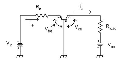
This circuit consists of an NPN transistor, forward biased emitter to  $base(V_{be})$  and reverse biased collector to base  $(V_{be})$ . Typically  $V_{be}$  is on the order of approximately .7 volts, so the current through  $R_e$ , is
