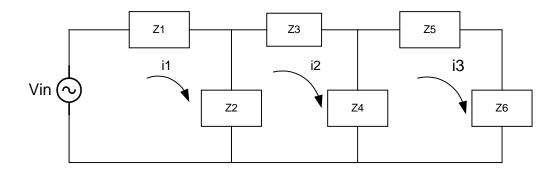
The procedure for any matrix greater than a  $2x^2$  as in the above example, is extended and modified slightly. In the case of the three loop circuit there a three columns and three rows;
