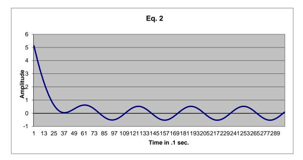
Again, please note that the output contains two distinct components: the transient response and the steady state response. The transient response is the time limited contribution of the impulse response (amplitude modified by the nature of the driver). The steady state response has the characteristics of the driver and continues until the drive is removed. All responses will contain these two components.
