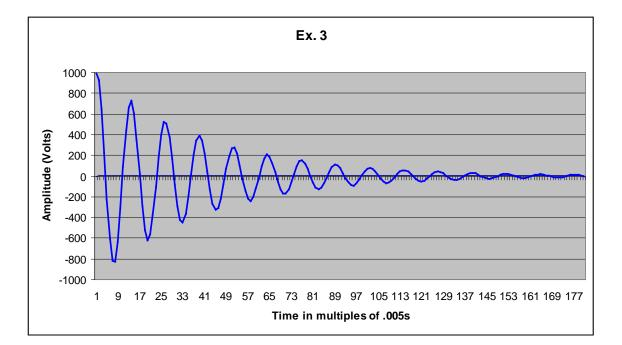
The tank exhibits a characteristic "ringing" that deteriorates over time in accordance with the system time constant. Task: identify the two components that determine the time constant; what is the theoretical result of a 0 ohm resistor? Question: is 0 ohm's possible under normal ambient conditions?
